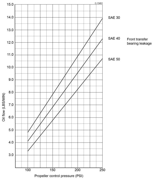
Figure C-4 Propeller Governor Oil Transfer Leakage
