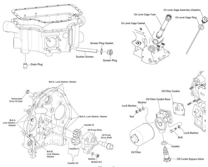
Figure 8 Lubrication System for LIO-360-B1G6 Engines
