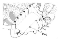
Figure 1 Plugs in the Induction System
