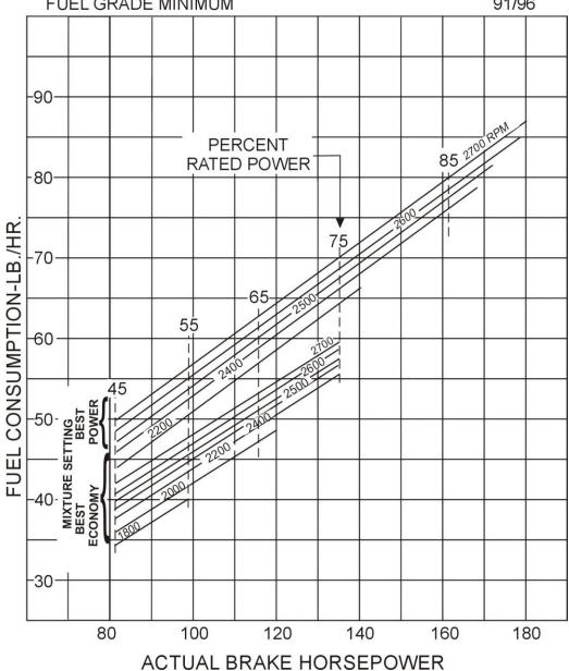
Figure C-3 Fuel Consumption vs. Actual Brake Horsepower
