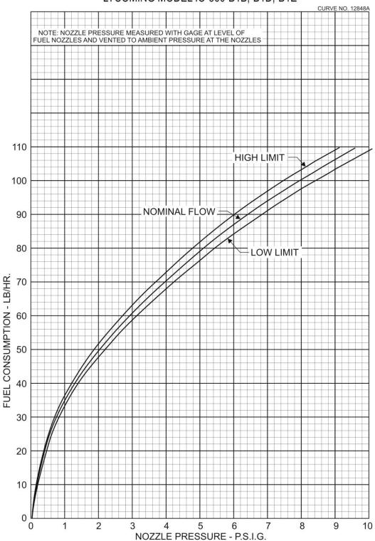
Figure C-2 Minimum Fuel Flow vs. Nozzle Pressure
