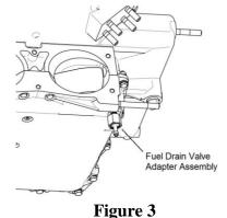
Fuel Drain Valve Adapter Assembly Installed in the Induction System
