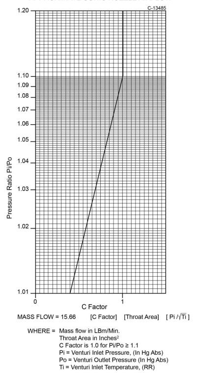
Figure A-3 Sonic Nozzle Airflow
