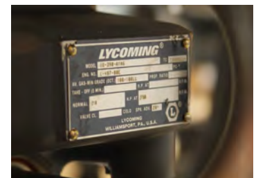
Figure 2 Engine Data Plate
