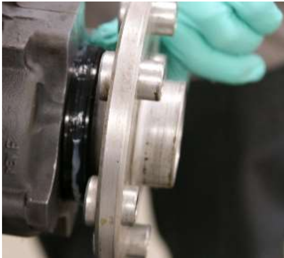
Figure 97 Work the Sealant Into the Seal Grooves
