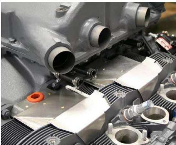
Figure 42 Placement of Intercylinder Baffle on Down Exhaust Engines
