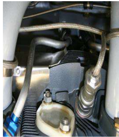
Figure 45 Loose Fit of Intercylinder Baffle
