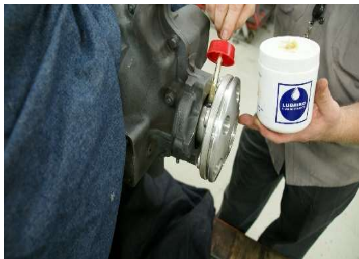
Figure 99 Apply Lubriko® M-6 Grease, Engine Oil or Equivalent to the Crankshaft
