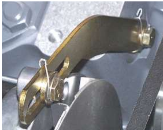
Figure 4 Safety Wire/Cable on Bolts of Alternator Adjusting Link
