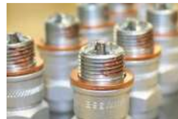
Figure 6 Copper-Based Anti-Seize Applied to Spark Plug Threads
