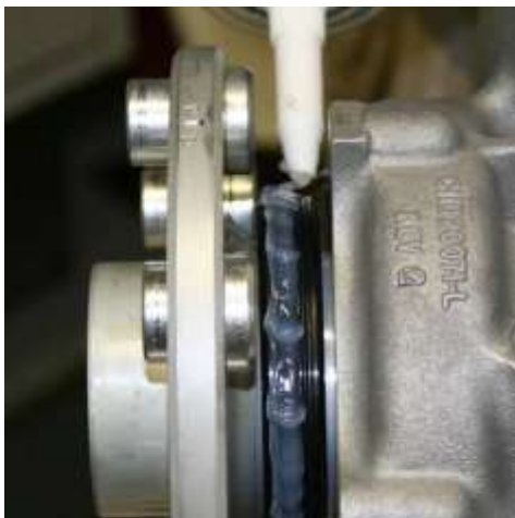
Figure 95 Apply the Sealant to the Oil Seal
