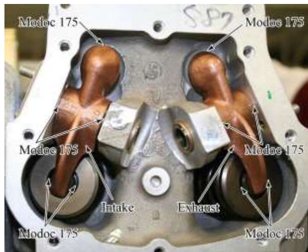
Figure 41 Valve Rocker Lubrication
