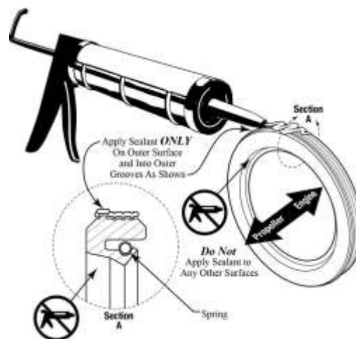
Figure 96 Apply the Sealant Only on the Outer Surface of the Oil Seal
