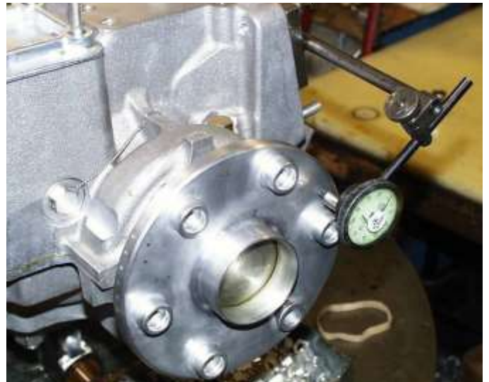
Figure 92 Crankshaft End Play Check
