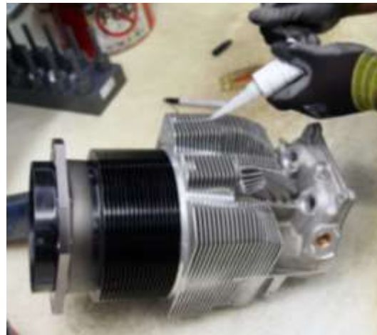
Figure A-4 Apply Adhesive
