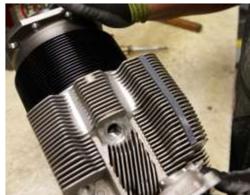
Figure A-5 Fin Stabilizer Installed on Cylinder
