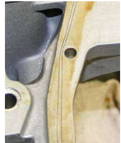
Figure 83 Placement of Silk Threads Along Inside Edge of Crankcase Flange
