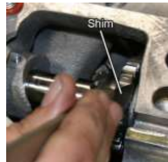
Figure 69 Shim Between Spacer and Crankcase – Backlash Check
