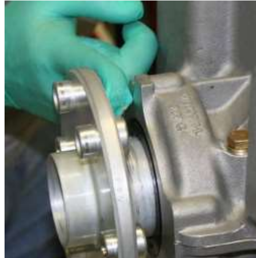
Figure 98 Spread the Excess Sealant
