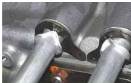
Figure 37 Correctly Aligned Shroud Tube Springs
