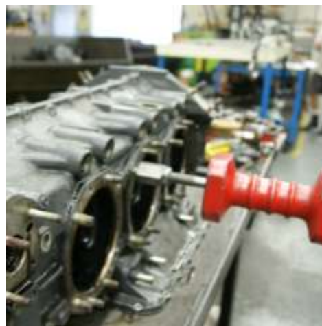
Figure 6 Strike the Slide Part of the Tool Against the Back of the Tool
