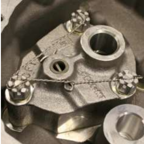
Figure 3 Safety Wire on the Oil Pump
