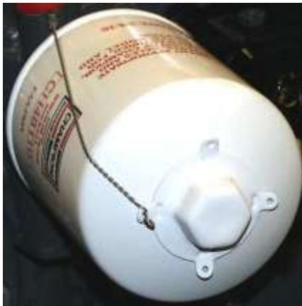
Figure 4 Safety Wire on Oil Filter
