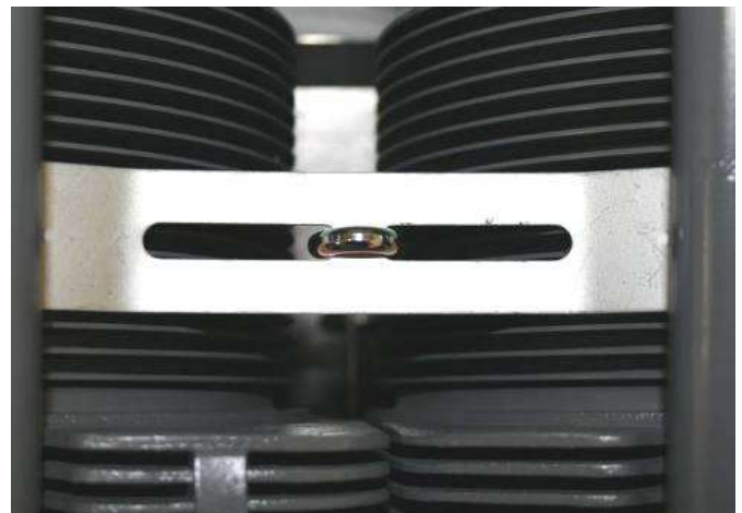
Figure 43 Intercylinder Baffle Installed on Three Fins
