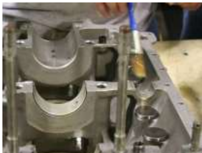
Figure 78 Lubricant Application to Camshaft Bearing Saddle in Crankcase Half
