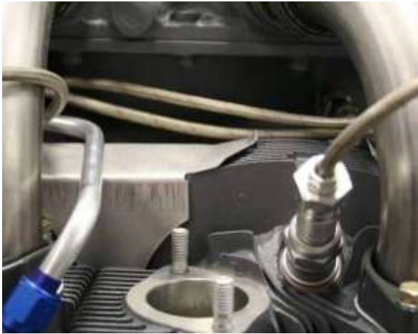
Figure 44 Correct Tight Fit of Intercylinder Baffle
