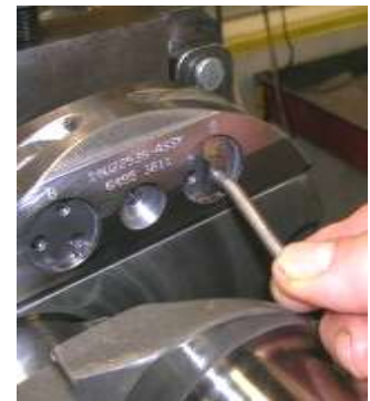
Figure 59 Insertion of Circlip Check Gage
