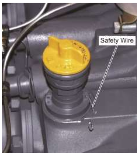
Figure 2 Safety Wire on the Oil Filler Extension
