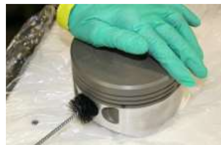
Figure 2 Cleaning the Piston Pin Bore with a Soft Bristle Non-Metallic Brush
