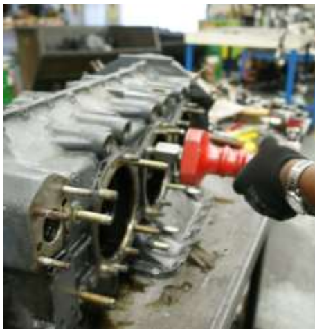
Figure 5 Attach the Slide-Hammer to a Base Stud
