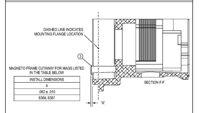
USE A CALIBRATED MEASURING DEVICE TO MEASURE DISTANCE "A", AS SHOWN IN CUTAWAY SECTION F-F. MAKE SURE THE FRAME SURFACE IS FREE OF CONTAMINANTS. ANY MEASUREMENT GREATER THAN .072 INCH OF ANY PART OF THE STOP PIN (3), THE MAGNETO SHOULD BE REMOVED FROM SERVICE AND RETURNED TO CHAMPION FOR WARRANTY.
